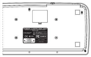
Figure 1.2: The battery compartment on the bottom side of the UMX25
